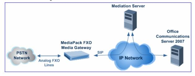
Figure 1-2: Network Architecture with PSTN Interface
